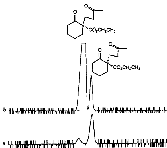
Fig. 2. Enantiomer separation of diketoesters 1(S) and 1(R) on the FS-Lipodex E chiral phase capillary column (140°C); (a) predominantly ( R )-enantiomer and (b) predominantly ( S )-enantiomer.
